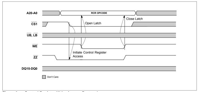
Figure 6 Control Register Write Access Protocol
