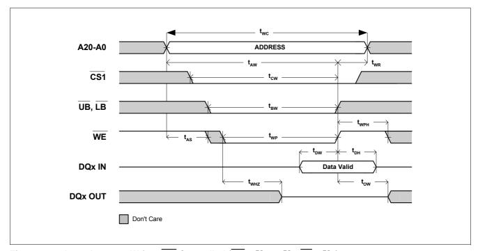
Figure 12 Asynchronous Write -  $\overline{\text{WE}}$  Controlled ( $\overline{\text{OE}} = V_{\text{IH}}$  or  $V_{\text{IL}}$ ,  $\overline{\text{ZZ}} = V_{\text{IH}}$ )
