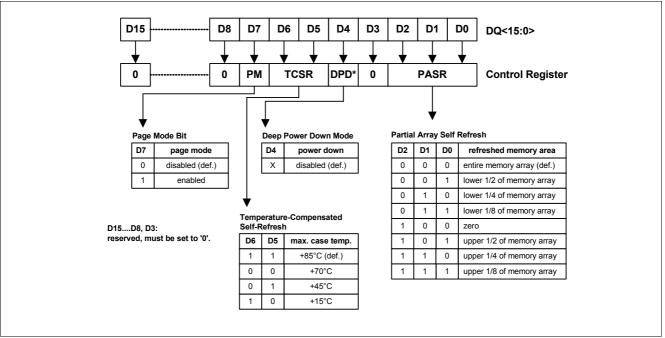
Figure 20 RCR Mapping in S/W Register Entry
