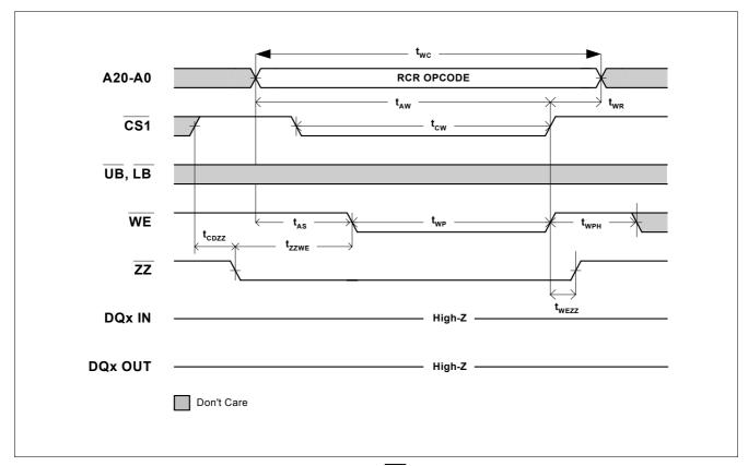
Figure 15 Asynchronous Write to Control Register ( $\overline{OE} = V_{IH}$  or  $V_{IL}$ )
