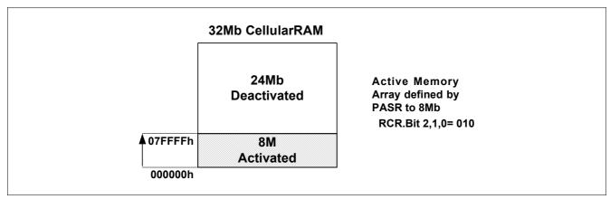
Figure 8 PASR Configuration Example
