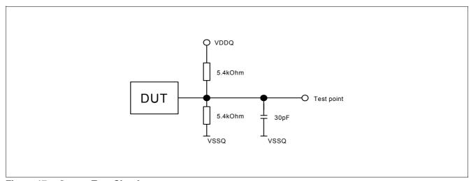
Figure 17 Output Test Circuit
