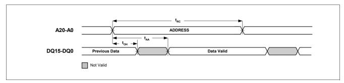
Figure 9 Asynchronous Read - Address Controlled ( $\overline{CS1} = \overline{OE} = V_{IL}$ ,  $\overline{WE} = V_{IH}$ ,  $\overline{UB}$  and/or  $\overline{LB} = V_{IL}$ ,  $\overline{ZZ} = V_{IH}$ )
