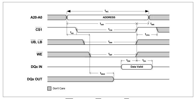
Figure 13 Asynchronous Write -  $\overline{CS1}$  Controlled ( $\overline{OE} = V_{IH}$  or  $V_{IL}$ ,  $\overline{ZZ} = V_{IH}$ )
