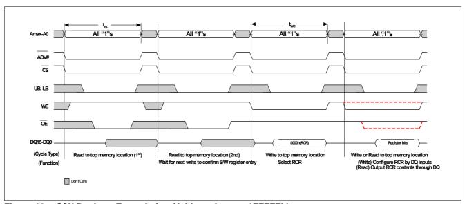
Figure 19 S/W Register Entry timing (Address input = 1FFFFFh)
