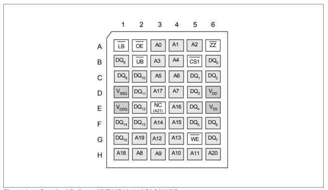
Figure 2 Standard Ballout - HYE18P32161AC(-/L)70/85
