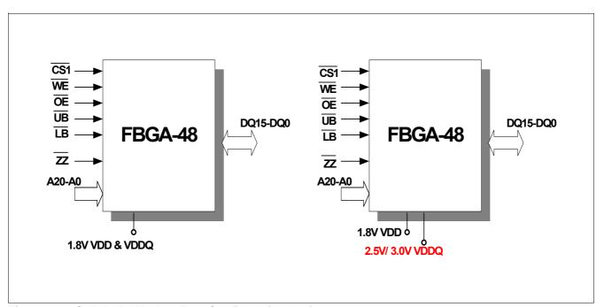
Figure 1 Cellular RAM - Interface Configuration Options
